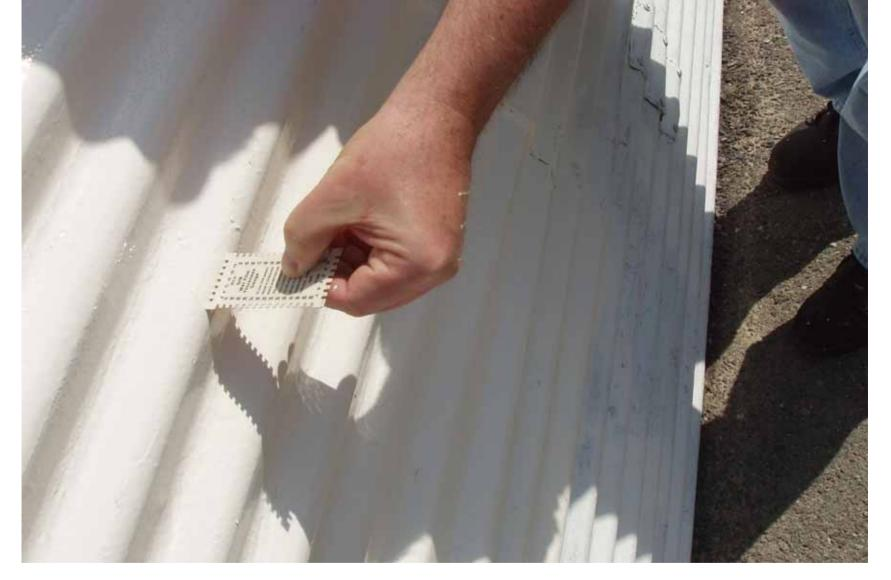
Wet Mil Gauge used to measure the applied coating thickness
