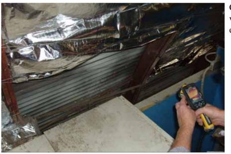
Comparing Interior Temperature of area that has a panel that was primed only with Metal Primer against the rest of the exterior wall coated with EnviroCoatings
