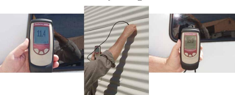
A series of Ultra-Sonic readings were taken around the Quonset Hut to measure dry film thickness.
